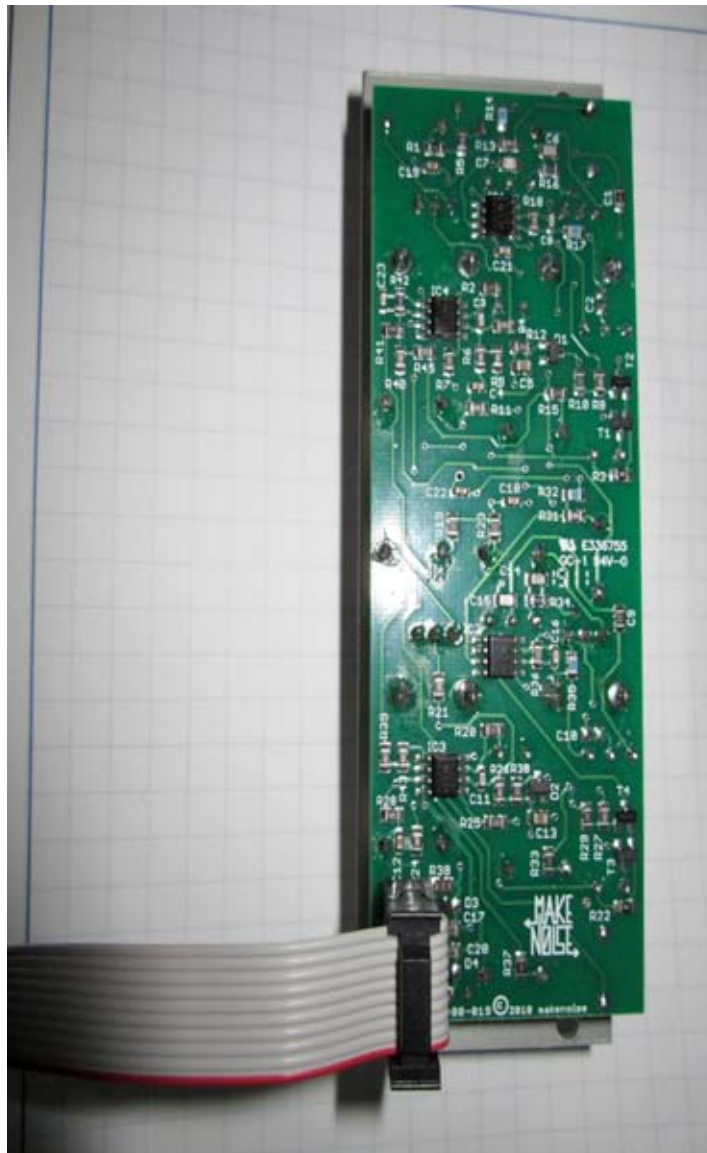
Proper installation of included power cable on module. Please note the RED BAND.
